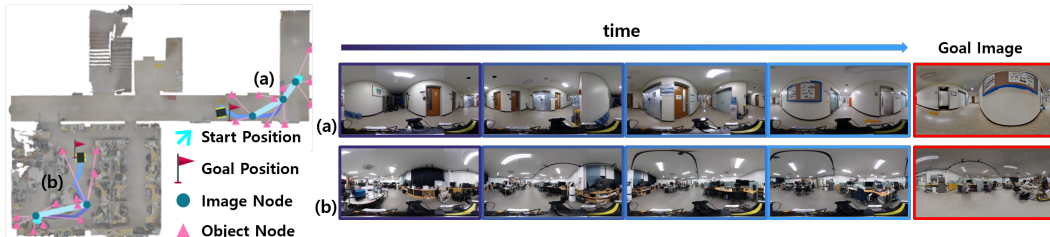
Figure 5: Visualization of the robot path on real environment. The color gradation represents the flow of time. The blue arrow symbolizes the starting point, and the red flag indicates the destination. An image node is represented by a blue circle, and an object node is represented by a pink triangle.
